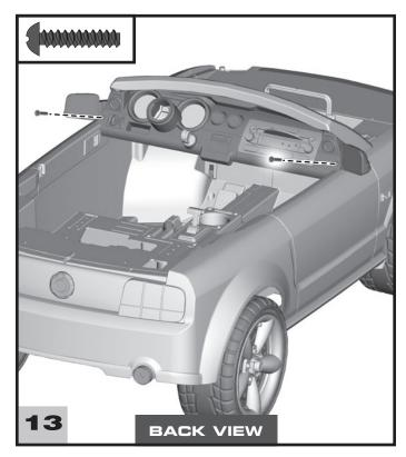
• Insert two black #8 x <sup>3</sup>/4" screws into the dash assembly as shown and tighten.
